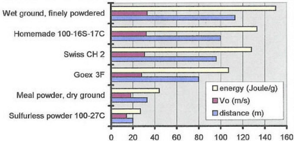
**Fig. 4:** Results fired with 1.00 gram of different powders
